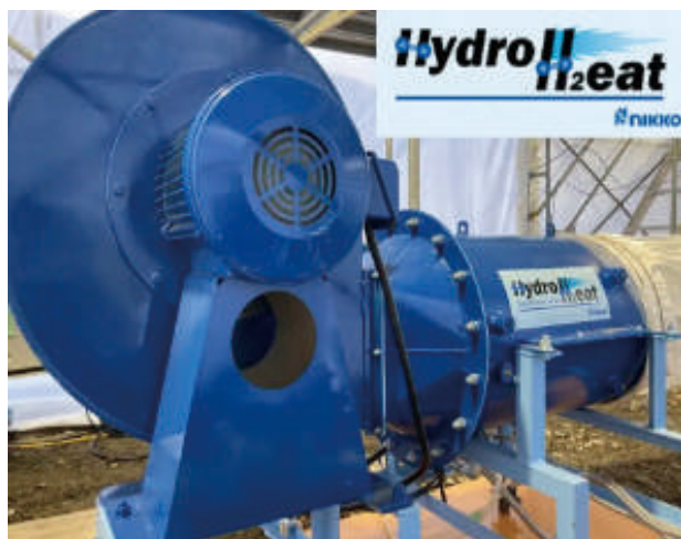
A hot-blast, direct-fired jet heater using hydrogen fuel
