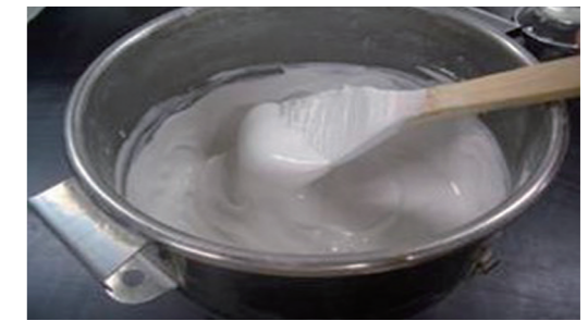
Photo 1: MC clay, at a W/S ratio of 140%, used in the experiment in this section 8)
